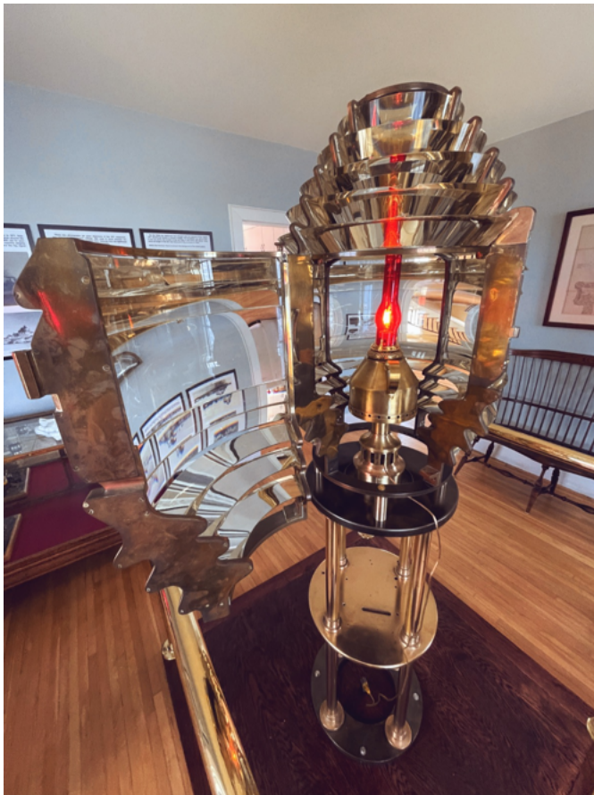
The completed Fresnel lens display with replica Funck lamp
