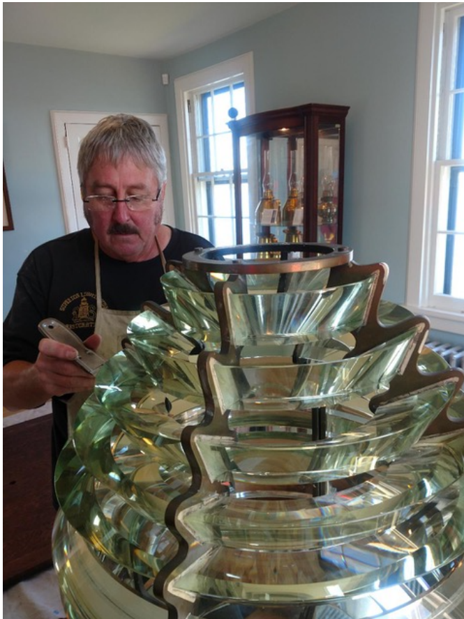
Lampist Kurt Fosburg cleans decades-old paint drips off the surface of the lens.
